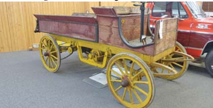
1910 Schmidt Model C Truck , chain drive, two cylinder engine. Manufactured in Crossing, Illinois, the Schmidt Brothers Co. produced half, three-quarter, and one-ton trucks. Public deliveries started in 1911
